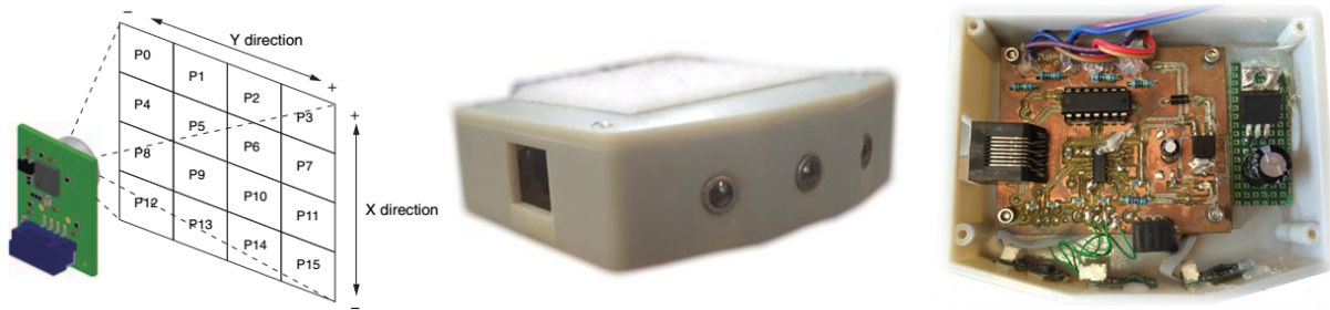
Figure 3. The detection area of the Omron D6T-44L [18]. The 3D printed box and circuitry for three thermal sensors.
